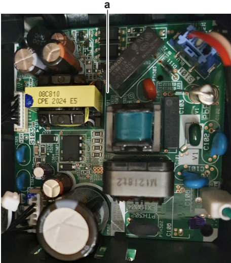
a Indoor unit power PCB
