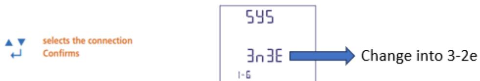
In case the energy meter is integrated with the Modbus communication network of the POL688 controller of the chiller unit, the Modbus parameters of the Nemo energy meter needs to be updated. It will be necessary to configure the address, transmission speed and parity bit on the energy meter corresponding to those on the chiller controller (POL688)
