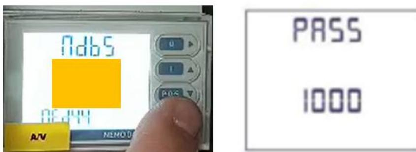
The “arrow” ► is used to move between the various digits, while ▲▼ is used to increment or decrement the numerical value of each digit. The ENTER key is used to confirm the password.
