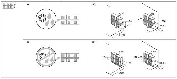
A1=>A2 (A1) If there is danger of drainage dripping and freezing between the upper and lower units...
