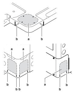
a Knockout hole for piping b Slit
