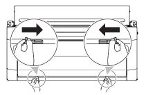
2 Remove the air filters. Holding the filter knob unhook the filter from the unit (2 places on each filter) and remove the filter.
