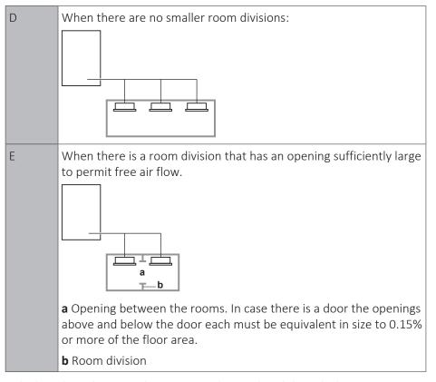
**3** Calculate the refrigerant density using the results of the calculations in steps 1 and 2 above. If the result of the above calculation exceeds the maximum concentration level, a ventilation opening to the adjacent room shall be made.
