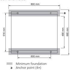
• Fasten the unit in place using four foundation bolts M12. It is best to screw in the foundation bolts until their length remains 20 mm above the foundation surface.
