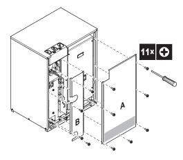
Once the front plate A is open, the electrical component box can be accessed. See "16.2.3 To open the electrical component box of the outdoor unit" [> 61].
