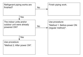
It is very important that all refrigerant piping work is done before the units (outdoor or indoor) are powered on. When the units are powered on, the expansion valves will initialise. This means that the valves will close.
