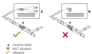
Make sure that the total length of the piping connected to the joint is absolute straight for more than 500 mm. Only if a straight field piping of more than 120 mm is connected, more than 500 mm of straight section can be ensured.
