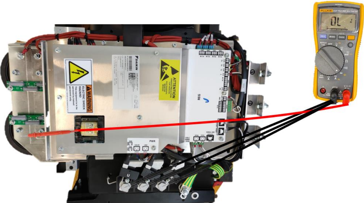
Figure 76 90 kW -120 kW DAE VFD - TOP IGBT Indirect polarization
