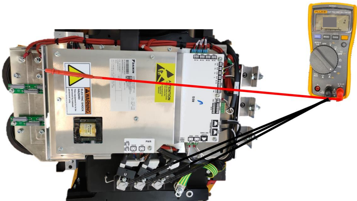
Figure 73 90 kW -120 kW DAE VFD – Bottom IGBT Direct polarization
