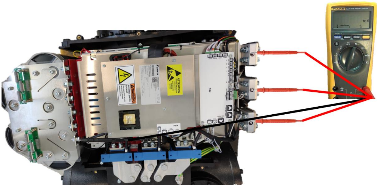
Figure 89 330 kW - 400 kW DAE VFD – TOP SCR Resistance direct polarization
