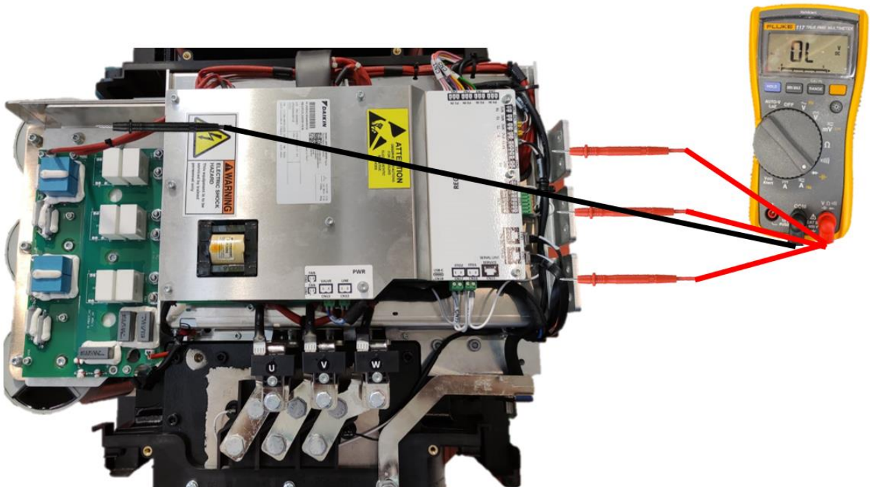
Figure 79 200 kW DAE VFD – Bottom SCR Indirect polarization
