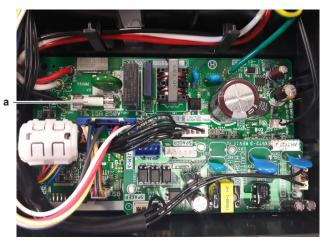
**2** To install a fuse on the indoor unit PCB, see "3.7.2 Repair procedures" [> 86].
