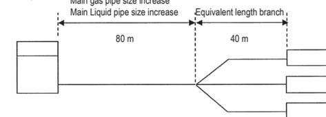
In the above case (Cooling) Overall equivalent length = 80 m x 1.0 + 40 m = 120 m
