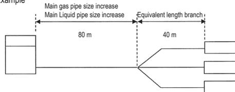
In the above case (Cooling) Overall equivalent length = 80 m x 1.0 + 40 m = 120 m
