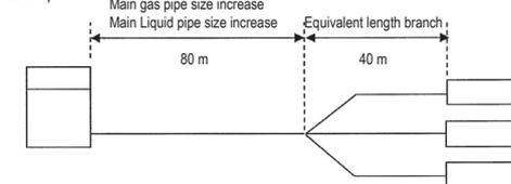
In the above case (Cooling) Overall equivalent length = 80 m x 1.0 + 40 m = 80 m
