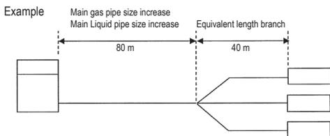
In the above case (for RXYQ38-44) (Cooling) Overall equivalent length = 80 m x 1.0 + 40 m = 120 m
