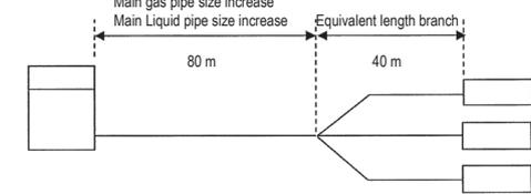
In the above case (Cooling) Overall equivalent length = 80 m x 0.5 + 40 m = 80 m
