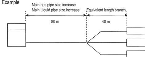
In the above case (Cooling) Overall equivalent length = 80 m x 0.5 + 40 m = 80 m
