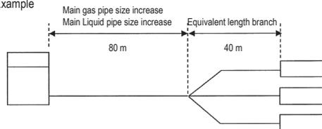
In the above case (Cooling) Overall equivalent length = 80 m x 0.5 + 40 m = 80 m
