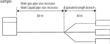
In the above case (Cooling) Overall equivalent length = 80 m x 1.0 + 40 m = 120 m
