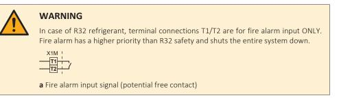
Remote control is available by transmission the external input to the terminals T1 and T2 on the terminal block for the user interface and the transmission wiring.
