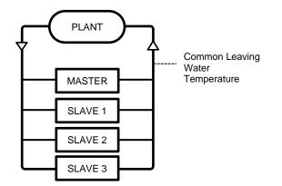
Master performs a so-called Partial control of each Slave unit in the system.
