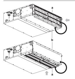
a Air filter holding plate with air filter(s)b Interchangeable plate
