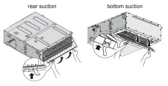
2 Clean the air filter. Use a vacuum cleaner or wash with water. If the air filter is very dirty, use a soft brush and neutral detergent.
