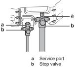
3 Recover gas and oil from the pinched piping by using a recovery unit
