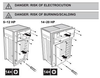
Once the front plates open, the electrical component box can be accessed. See "14.2.2 To open the electrical component box of the outdoor unit" [> 28].
