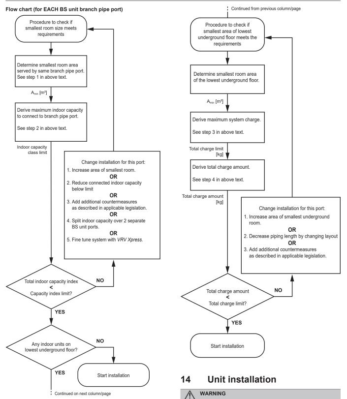
The installation MUST comply with the requirements that apply to this R32 equipment. For more information, see "13 Special requirements for R32 units" [> 21].
