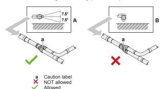
Make sure that the total length of the piping connected to the joint is absolute straight for more than 500 mm. Only if a straight field piping of more than 120 mm is connected, more than 500 mm of straight section can be ensured.
