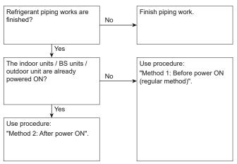
It is very important that all refrigerant piping work is done before the units (outdoor, BS unit or indoor) are powered on. When the units are powered on, the expansion valves will initialise. This means that the valves will close.
