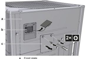
b Main PCB with 3 7-segment displays and 3 push buttons
