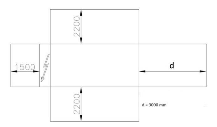
For single unit installation in proximity of a wall the following indications are recommended:
