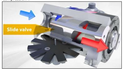
To obtain the best possible efficiency at every working condition, Daikin compressors can adjust the geometry of the discharge port according to the real operating conditions slightly delaying or anticipating the discharge phase of the refrigerant minimizing the losses for under or over compression and so enhancing the efficiency. This is possible thanks to a sliding valve.
