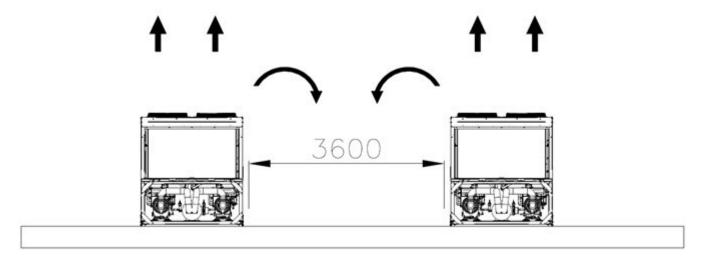
In case of two units installed in a compound contact local Daikin representative to evaluate possible arrangements. For multiple units' installation, it is recommended to install the units in a single row as shown in the below picture
