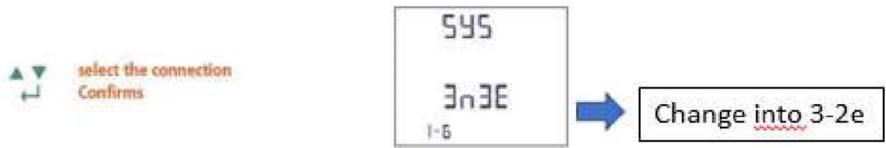
In case the energy meter is integrated in the modbus communication network of the POL687 controller of the chiller unit , the modbus parameters of the Nemo energy meter needs to be updated. It will be necessary to configure the address, transmission speed and parity bit on the energy meter corresponding to those on the chiller controller (POL 687).
