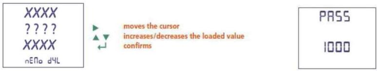
The "arrow" ▶ is used to move between the various digits, while ▲ ▼ is used to increment or decrement the numerical value of each digit. The ENTER key is used to confirm the password.
