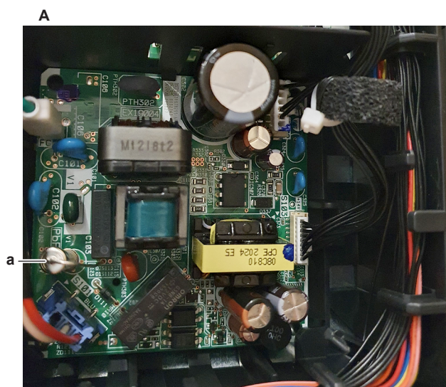
A Wall mounted indoor unit ATXM20R + CTXM15R a Fuse F1U
