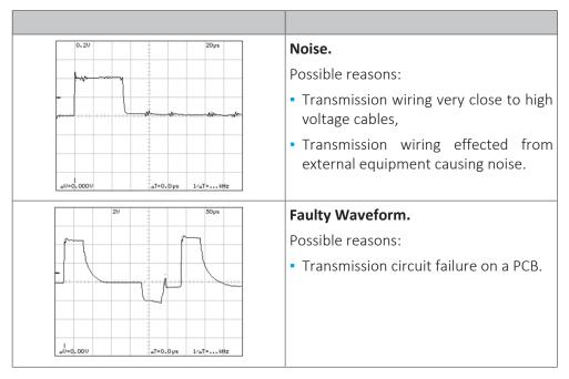
After checking and correcting possible causes of F1-F2 transmission problems, perform a communication reset (see "4.1.2 Repair procedures" [▶ 304]).
