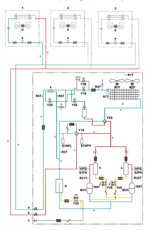
Indoor unit 1: Operation ON, Thermo ON, Fan ON, Expansion valve: normal control **Indoor unit 2:** Operation OFF, Fan OFF, Expansion valve: average subcool control
