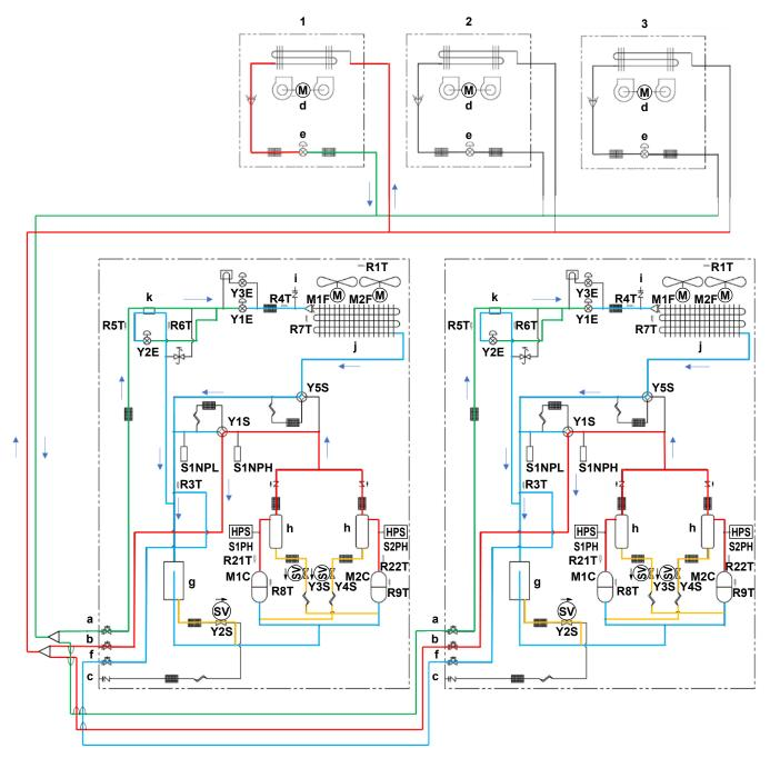
Operation ON, Thermo ON, Fan ON, Expansion valve: normal control Operation OFF, Fan OFF, Expansion valve: average subcool ontrol Indoor unit 2: Indoor unit 3: Operation ON, Thermo OFF, Fan ON, average subcool control
