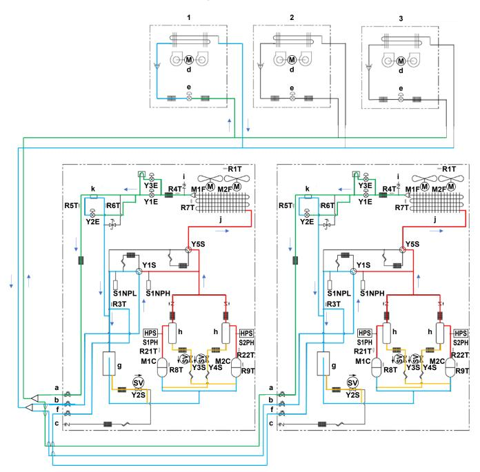
Indoor unit 1: Operation ON, Thermo ON, Fan ON, Expansion valve: normal control
