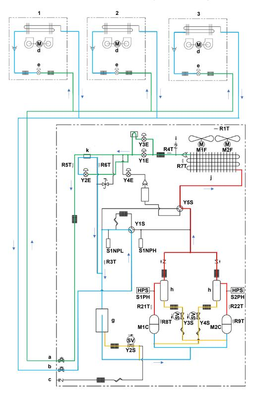
**Indoor unit 1:** Operation ON, Thermo ON, Fan ON, Expansion valve: normal control
