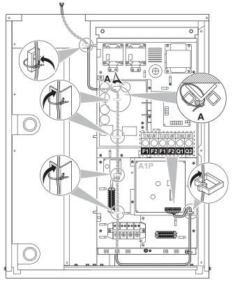
Fix to the indicated plastic brackets (factory installed).
