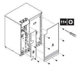
Once the front plate A is open, the electrical component box can be accessed. See "17.2.3 To open the electrical component box of the outdoor unit" [> 61].
