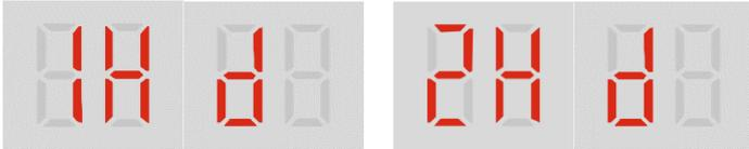
In the error code, 'y' is a placeholder for the address (1, 2) of the slave unit with the error.
