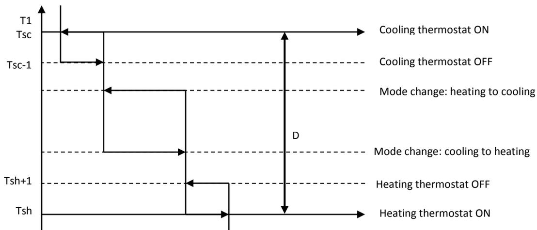
Tsc: Cooling target set temperature,  $26^{\circ}\text{C}$  default
