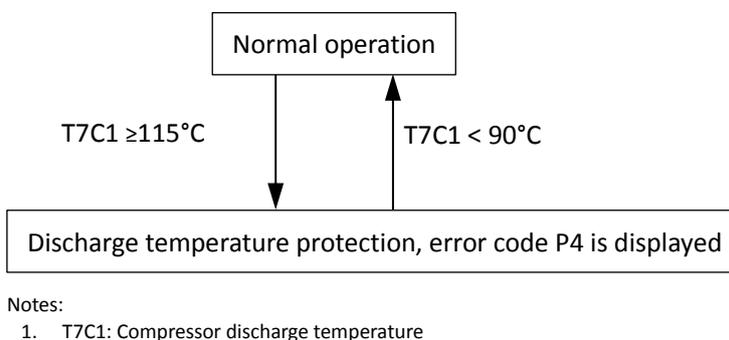
When the discharge temperature rises above 115°C the system displays P4 protection and all units stop running. When P4 protection occurs 3 times in 100 minutes, the H6 error is displayed. When an H6 error occurs, a manual system restart is required before the system can resume operation.
