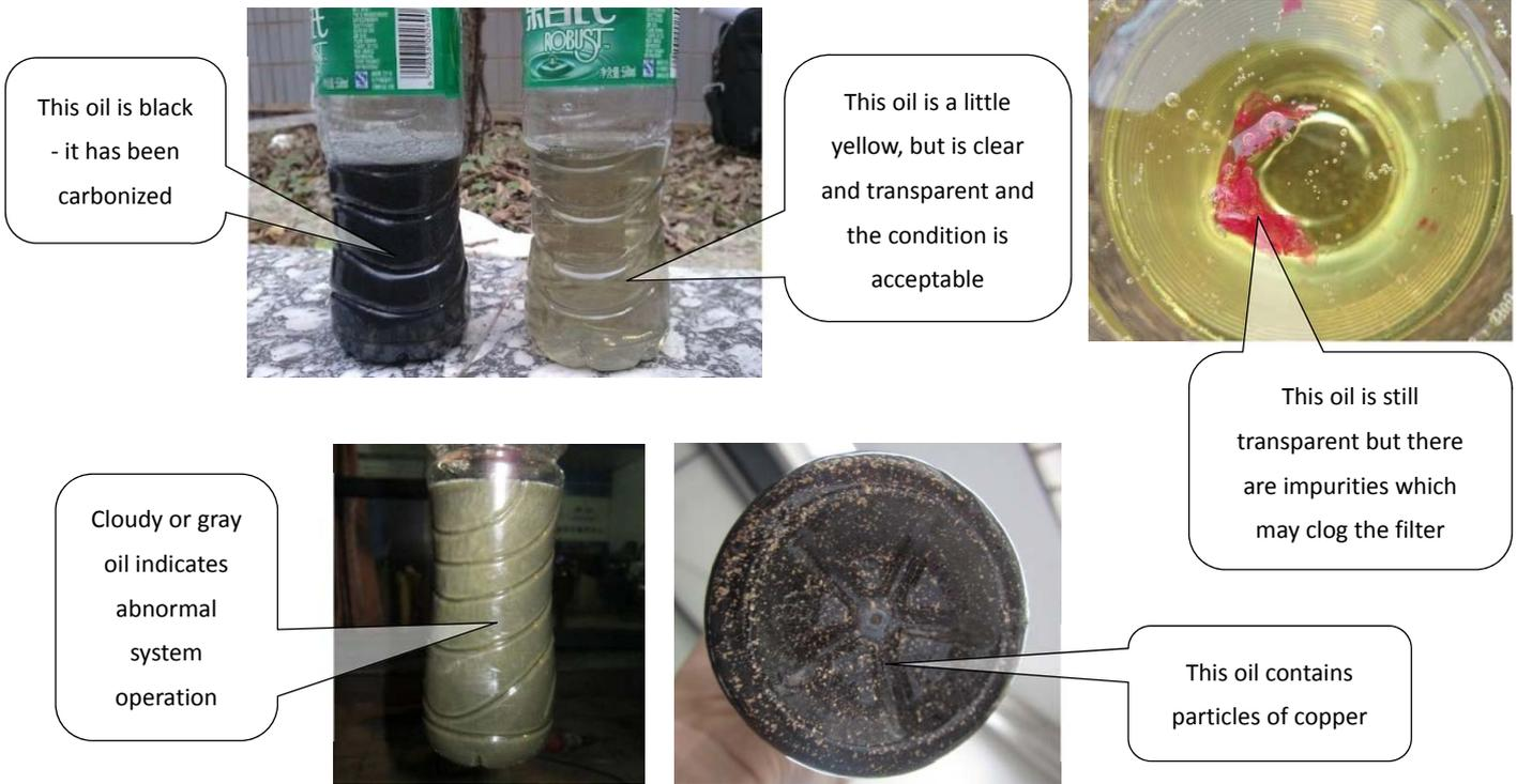
Figure 6-2.11: Effects of spoiled compressor oil
