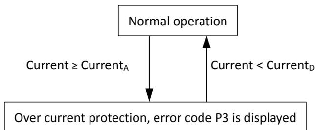
Table 3-6.1: Current limitation for compressor inverter modules
