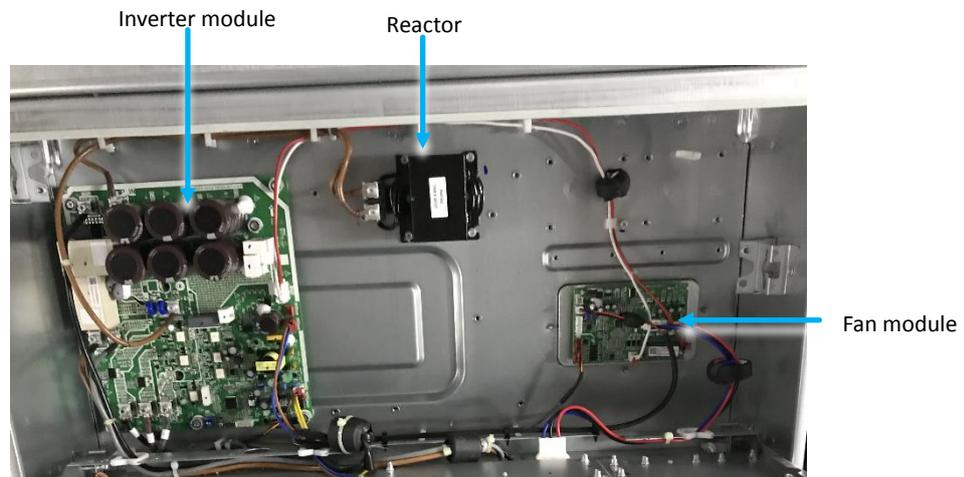
Figure 5-1.3: 14-20HP top layer of electric control box
