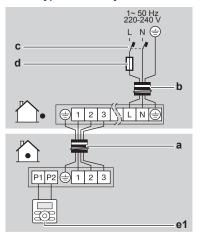
Simultaneous operation system. 1 user interface controls 2 indoor units (indoor units operate simultaneously)
