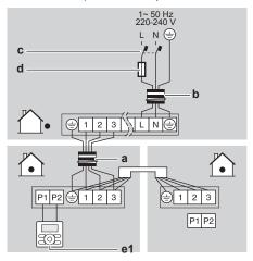
Group control. 1 user interface controls up to 16 indoor units (all indoor units operate according to the user interface).
