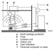
In places with weak reception, keep distances of 3 m or more to avoid electromagnetic disturbance of other equipment and use conduit tubes for power and transmission lines.
