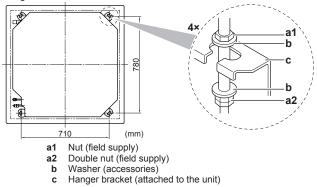
• Paper pattern for installation (upper part of the packing). Use the paper pattern to determine the correct horizontal positioning. It contains the necessary dimensions and centers. You can attach the paper pattern to the unit.
