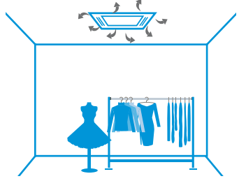
Air distribution with a dusty filter
