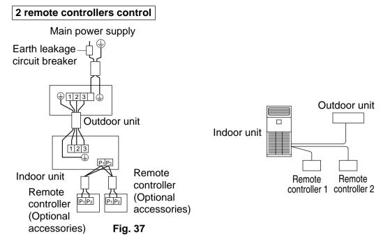
Two remote controllers control (Controlling 1 indoor unit by 2 remote controllers)
