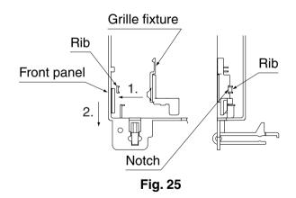
3. Fix the control panel on the back side of the front panel.
