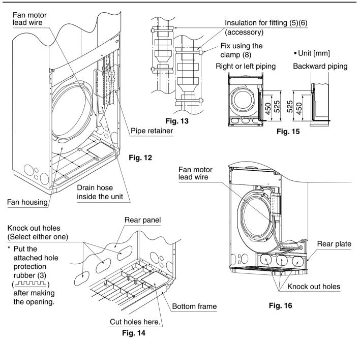
• After the refrigerant piping and electrical wiring work is completed, hold the refrigerant piping, the indoor unit drain hose, the wiring connecting the indoor and outdoor units and the earth wire with the piping retainer plate (**Refer to Fig. 12**). During this work the refrigerant piping entering into the indoor unit may come in contact with the suction grille. Therefore, make sure not to extend the refrigerant piping from the piping retainer plate.
