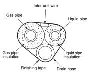
2. Be sure to insulate both the gas and liquid piping and to provide insulation dimensions as below.
